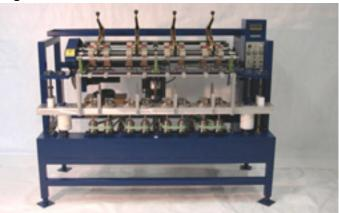
Pictured above is a Belfast mini mills 8 spindle spinner, equipment similar to this is what is being considered.
